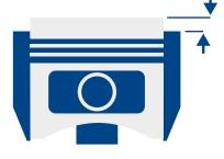
According to the measurements obtained, we might select the right cylinder head gasket from the next index.
